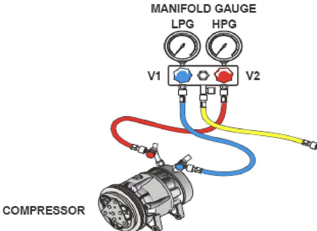
**Figure 17:** Installing Manifold Gauge into the System.
