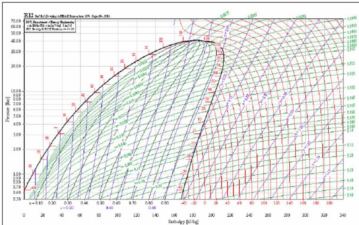
**Figure 6: Pressure – Enthalpy Diagram for R-12.**
