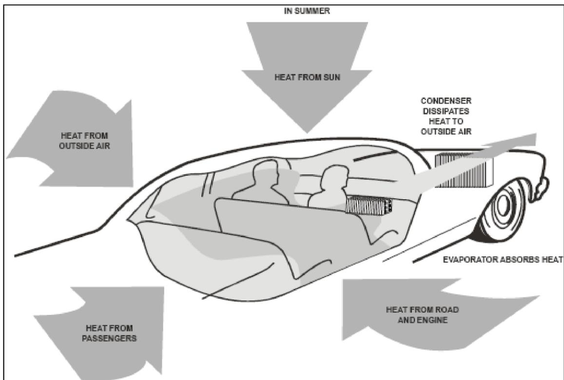
**Figure 1:** Absorb and Releasing the Heat in Automotive Air Conditioning Operation.
