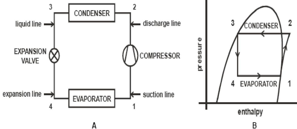
**Figure 4:** Vapor Compression System Schematic and refrigeration Cycle pressure-Enthalpy Diagram
