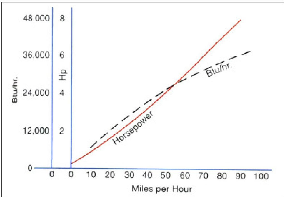
**Fig. 3:** Curves show relationship between car speed, heat load, and horsepower required to drive air conditioning system.
