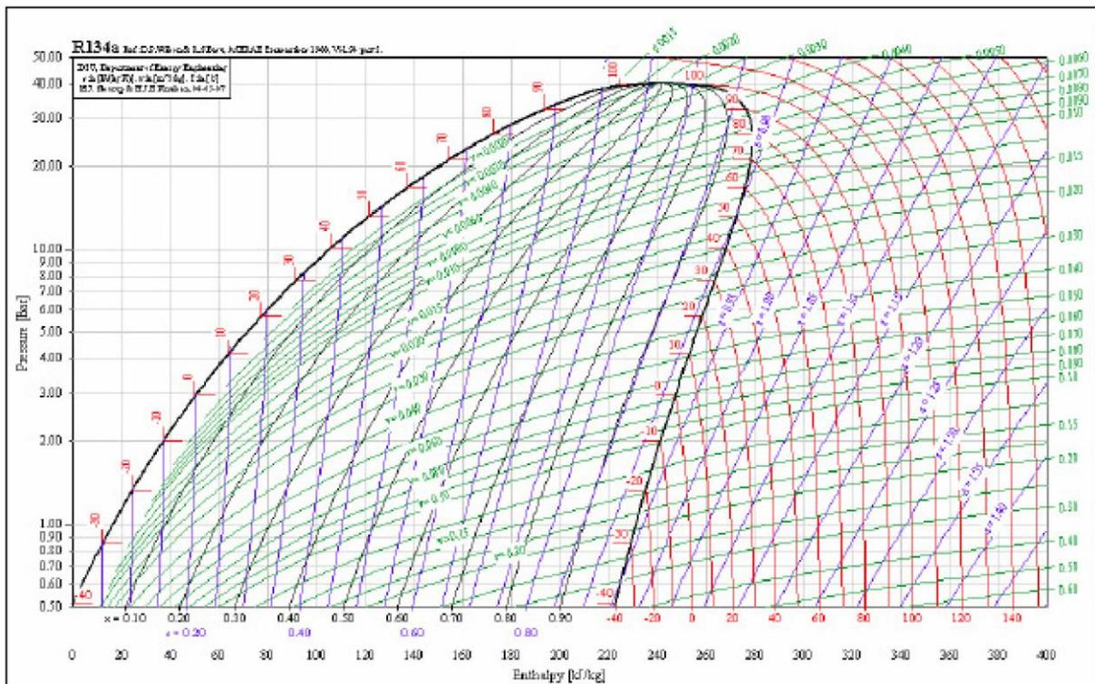
**Figure 8:** Pressure – Enthalpy Diagram for R-134a.
