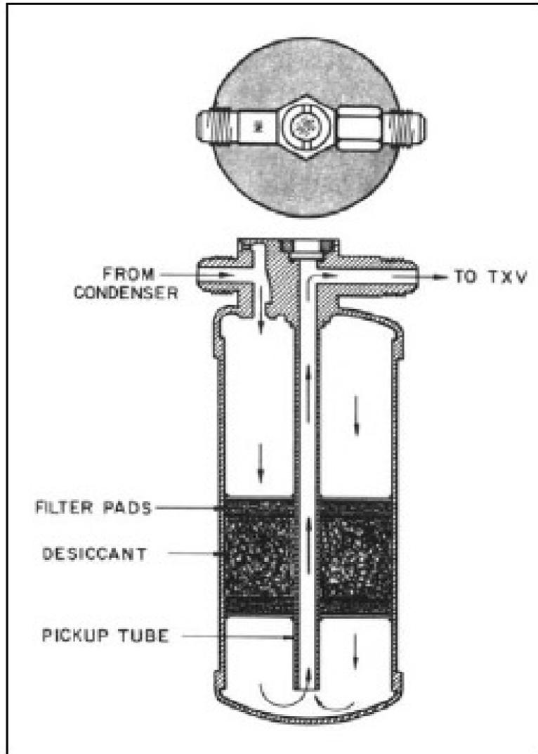
**Figure 12: Receiver Drier**
