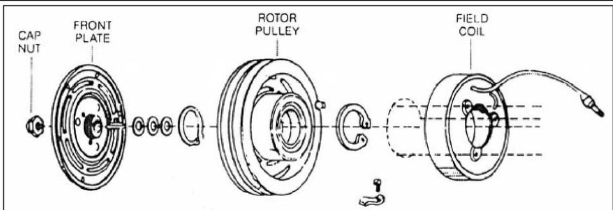
**Figure 10:** Internal View of The Compressor Magnetic Clutch.
