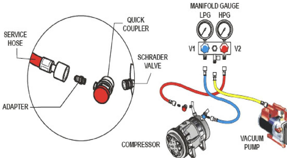
**Figure 16:** Connections parts for installing manifold gauge into the system and purging the air in the service hoses.
