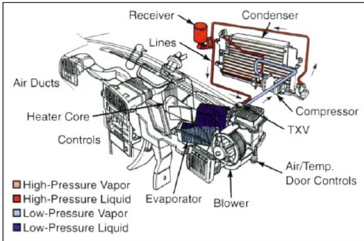
**Figure 2:** Typical Automotive Air Conditioning System that use a TXV and Receiver Drier.
