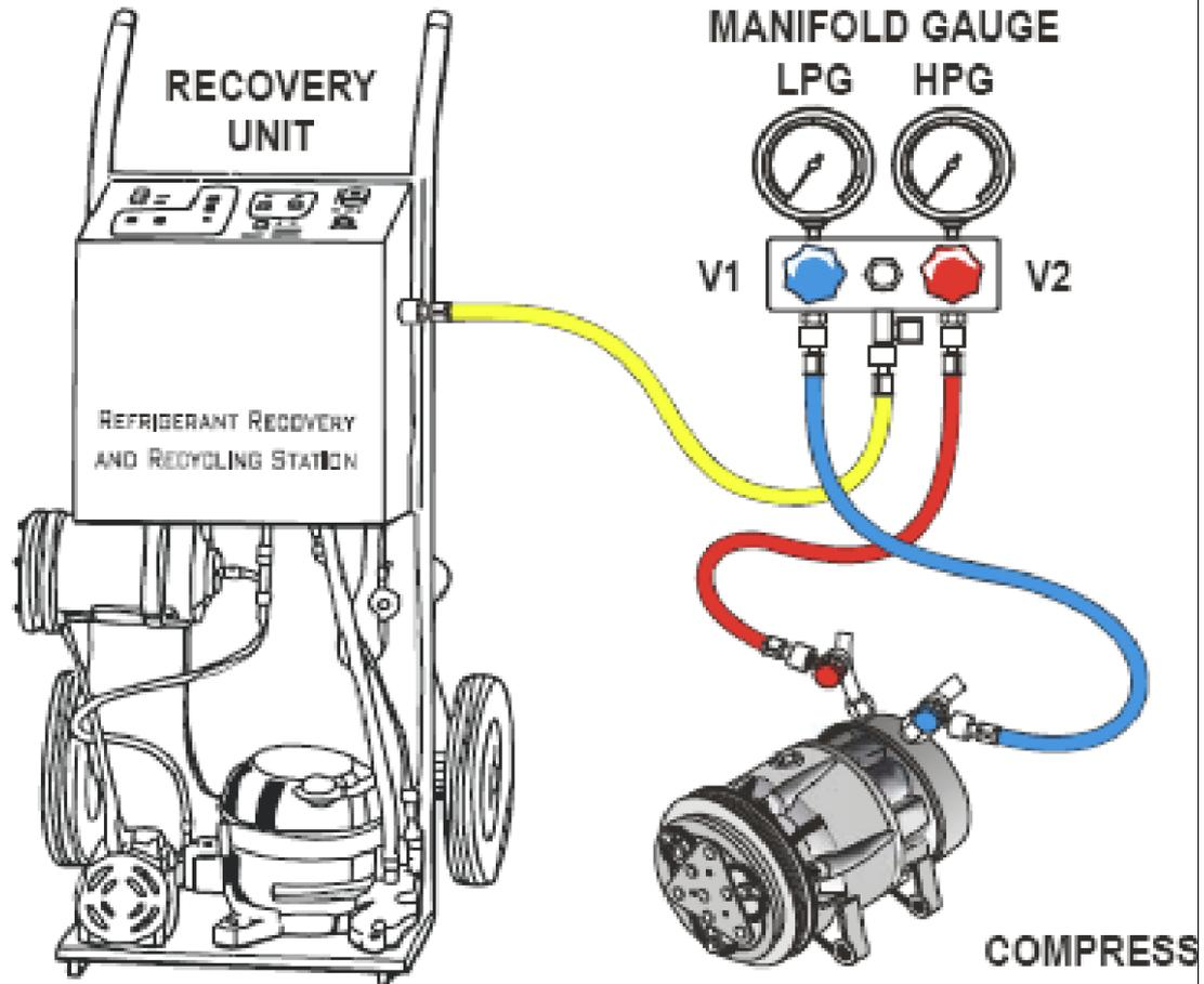
**Figure 18:** Connecting recovery unit to manifold gauge.
