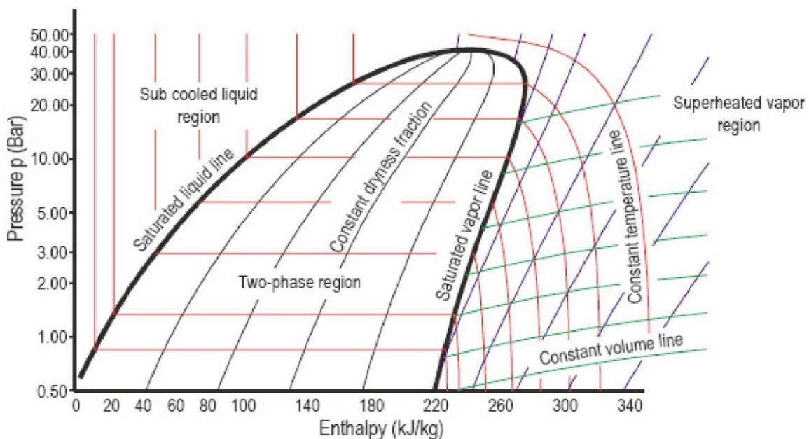
**Figure 5:** Skeleton of Pressure-Enthalpy Diagram.
