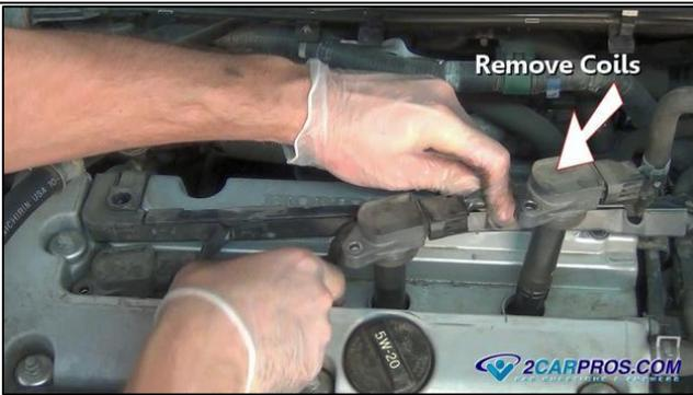
4. Inspect THE condition of the coil for any crack, burn or etc.
