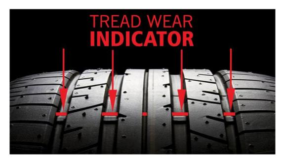
Figure 9: Thread wear indicator
