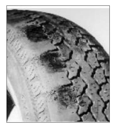
Figure 7: Effect of weak suspension on tyre
