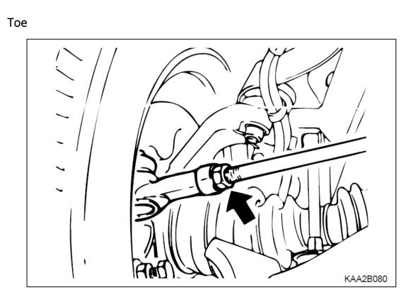
Figure 12 : Loosen the tie rod end lock nuts to adjust toe angle
