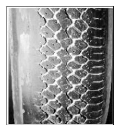
Figure 5: Tyre Wear On One Side
