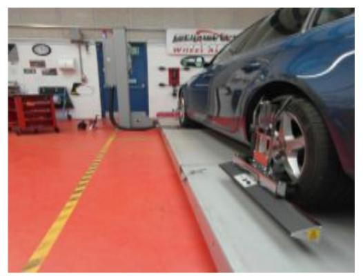
• Begin the alignment procedure by first driving the vehicle onto the alignment rack as straight as possible.
