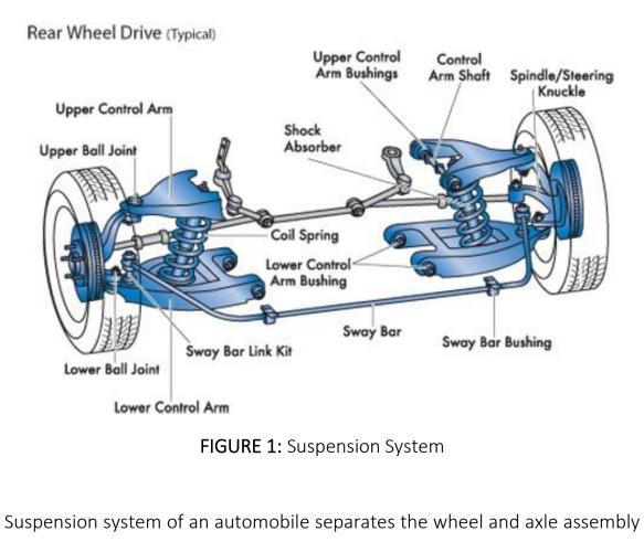
of the automobile from its body. Main function of the suspension system is to
