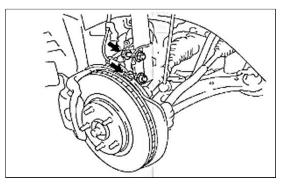
Figure 11 : Replace knuckle nut with camber bolt
