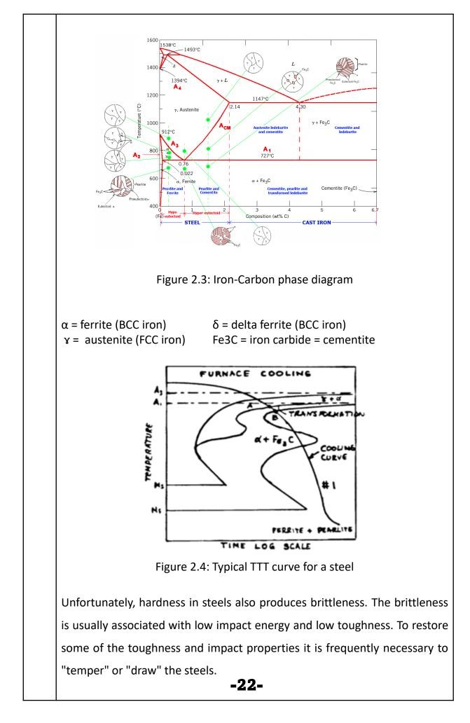
This is accomplished by heating the steel to a temperature between 260°C and 540°C. Tempering removes some of the internal stresses and introduces recovery processes in the steel without a large decrease in hardness or strength.
