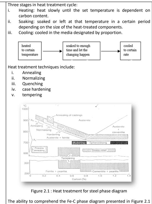
The ability to comprehend the Fe-C phase diagram presented in Figure 2.1 is based on understanding heat treatment of steels. Eutectoid steel has a C content of 0.76 percent by weight. Steel with a carbon percentage of less than 0.76 wt% C is hypoeutectoid, while steel with a carbon content of more than 0.76 wt% C is hypereutectoid. Austenite has a face-centered-cubic (FCC) region, while ferrite has a body-centered-cubic (BCC) zone (BCC).
