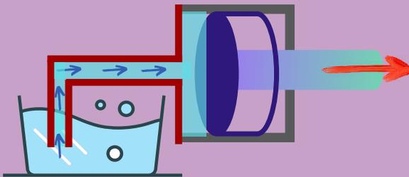
which use hydraulic power to enable mechanical operation, is mainly composed of a cylinder or fluid motor.
