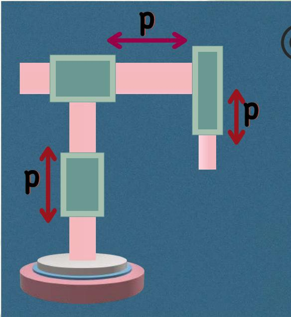
Three linear joints are used in the design of the cartesian robots. The cartesian plane, which includes X, Y, and Z, has these joints. Additionally, these robots could have a connected wrist with simpler rotating joints. Another name for this particular type of robot is rectilinear or gantry.
