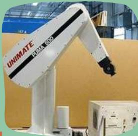
Unimation placed a PUMA (Programmable Universal Machine for Automation) robot in a GM plant. The importance of vision, tactile sense, and intelligent control becomes clear for research areas as the result.
