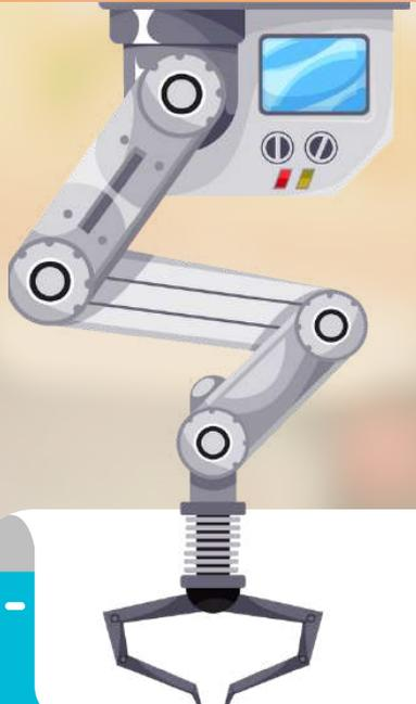
An end effector is a robotic device used to interact with the environment. It is located at the end of a robotic arm. It is an apparatus that is fastened to the manipulator's wrist.
