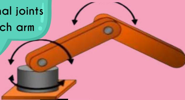
This robot that offers planar compliance and has two parallel rotary joints.
