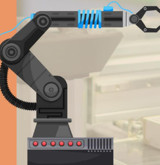
Its work envelope is the area that the robot's end effector can access. The goal is to grab, hoist, move, manipulate, or work on the work item.
