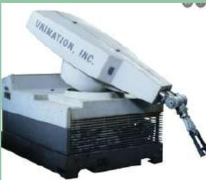
Starting at the General Motors plant, the first industrial robot from Unimate from Unimation was inspired for the plant as a casting machine unloading machine.
