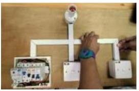
• Turn on the switch at main switch, residual current circuit and miniature circuit breaker. Finally, turn on the two-way switches to light up the lamp
