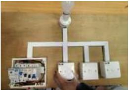
• Turn on the switch at main switch, residual current circuit and miniature circuit breaker. Finally, turn on the switches to light up the lamp
