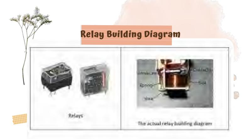
A simple electromagnetic relay consists of a coil of wire wrapped around a soft iron core , an iron yoke which provides a low reluctance path for magnetic flux, a movable iron armature, and one or more sets of contacts. The armature is hinged to the yoke and mechanically linked to one or more sets of moving contacts. It is held in place by a spring so that when the relay is de-energized there is an air gap in the magnetic circuit.
