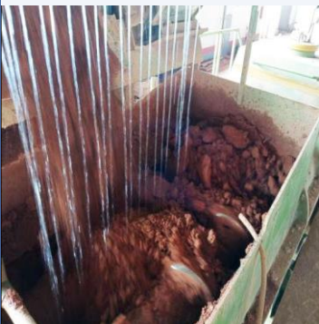
Clay Grinding and Mixing
