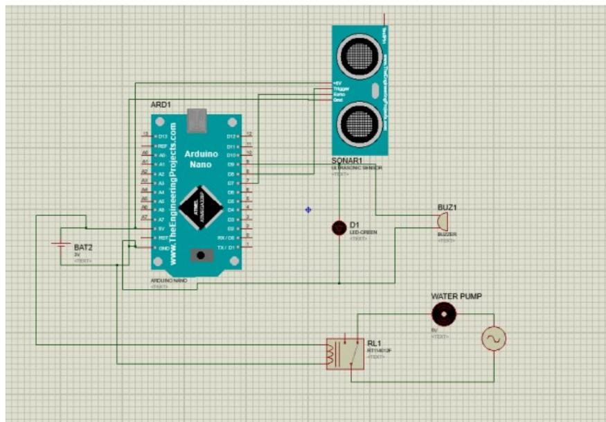
Figure 3. The system schematic
