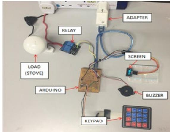
Figure 1. Circuit implementation on Breadboard
