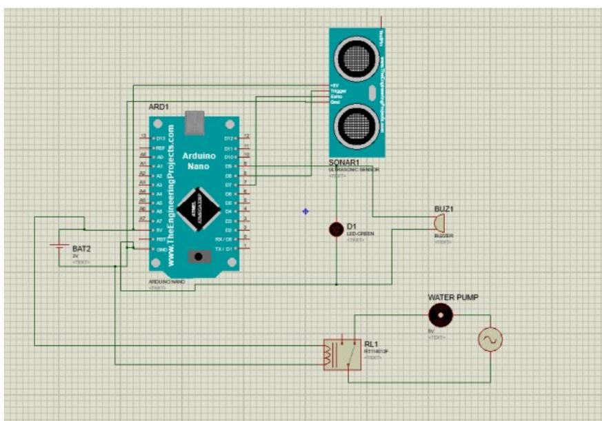
Figure 3. The system schematic
