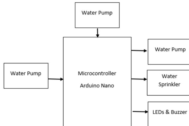
Figure 1. The rainwater system using ultrasonic sensor block diagram
