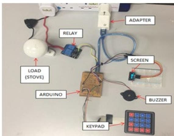
Figure 1. Circuit implementation on Breadboard
