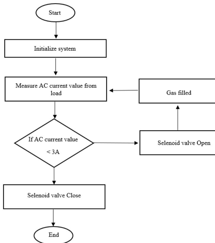
Figure 2. Block diagram of this project
